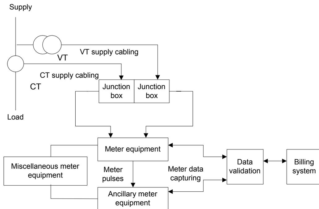
Figure 1 — Metering system diagram
