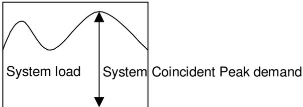
If the System Coincident Peak demand values are not available, calculate the Coincident Peak demand for each load by using the Bary load/coincident factor graph. A copy of the Bary load/coincident factor curve is attached hereto. The non-coincident load is multiplied with the Bary coincident factor to determine the coincident load.
