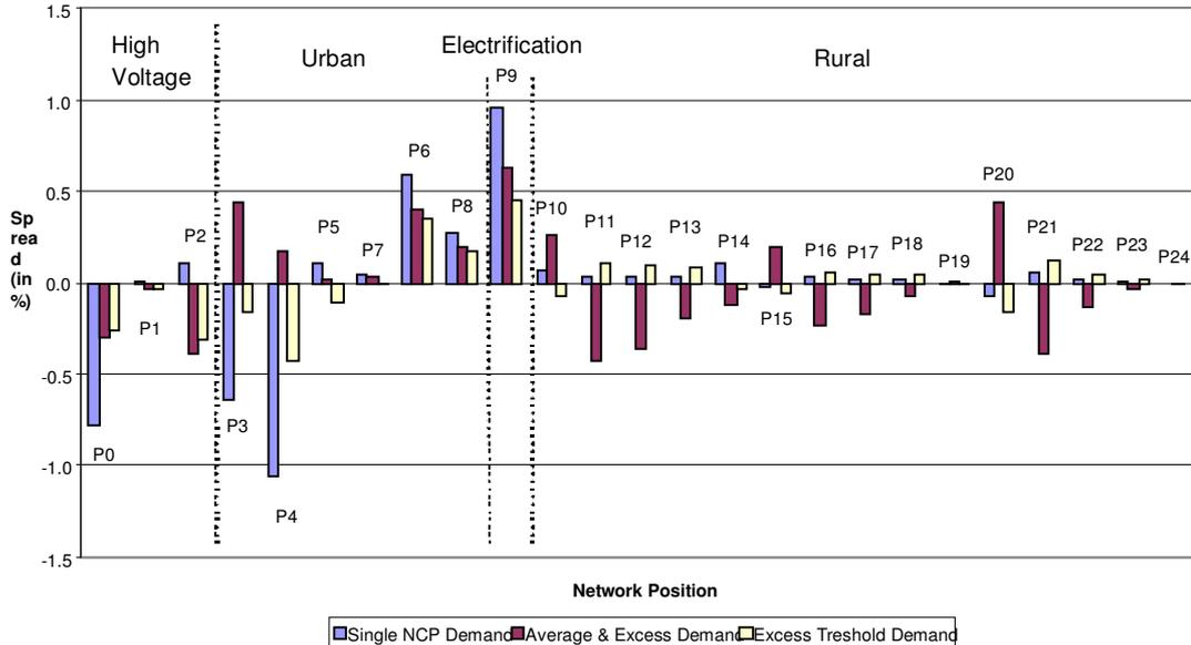
Figure C.1 – Spreads per Customer Group as compared to the current Eskom Method
