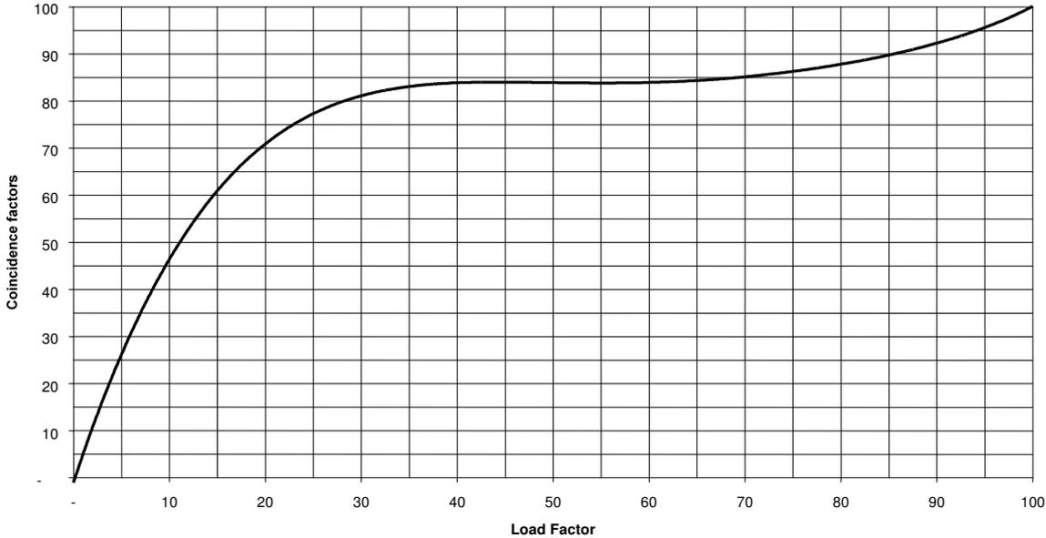
This graph is used to determine the simultaneous or co-incident demand for customers where only the non-coincident demand is measured or estimated. It is used in the Average & Excess methodology
