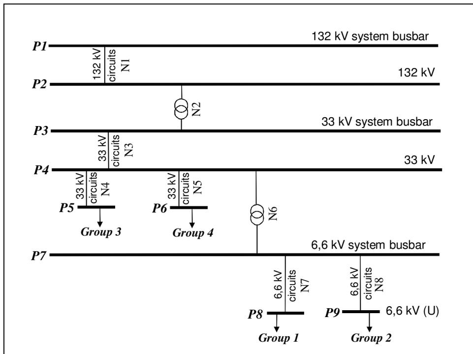
**Figure F.1 – The RND indicating the loads of each Customer Group, the network and the location of the loads. P1 to P8 indicate different positions in the RND**
